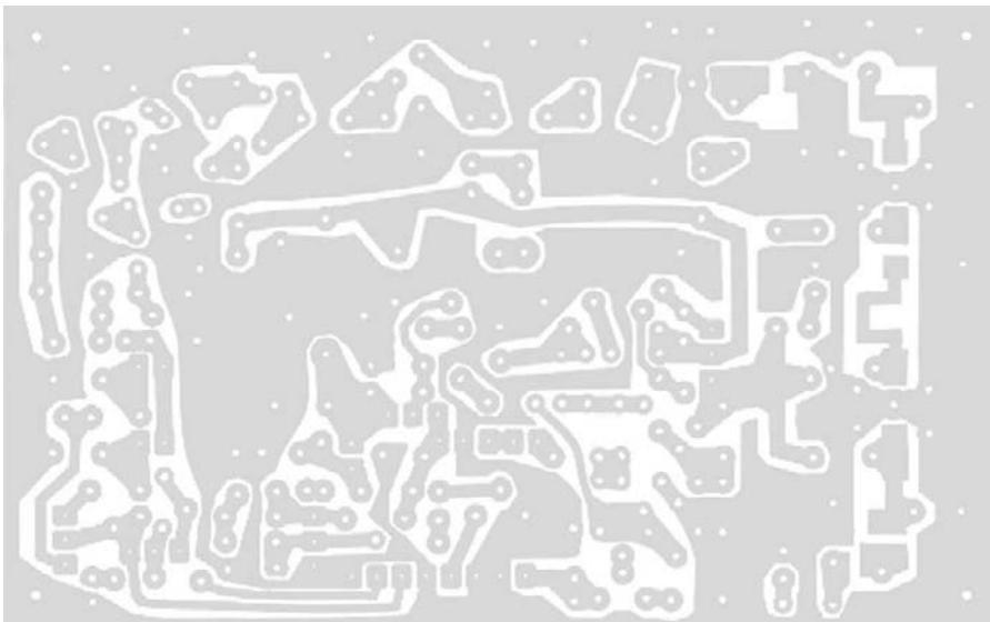
Figure 13-8 Solder Side of the PC Board for the ATV12-1300 MKII
