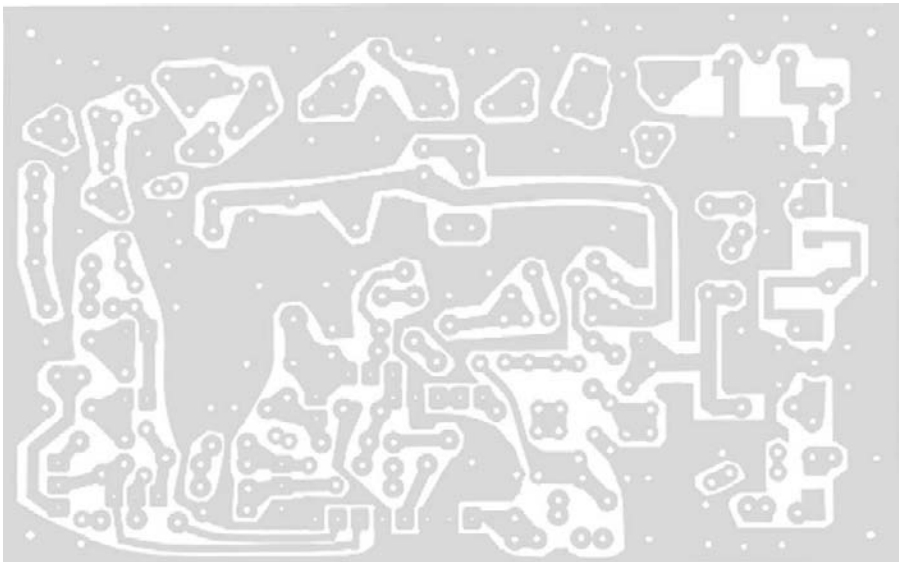
Figure 13-6 Solder Side of the PC Board for the ATV12-900 MKII
